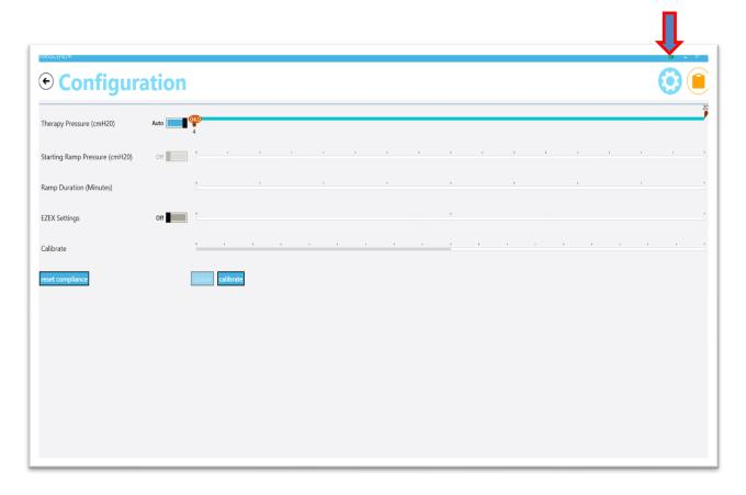
The Configuration area is used to adjust various settings on the device. Some features, such as the Therapy Pressure and Calibration are clinician settings and are only available with a password. You can, however, adjust the Starting Ramp Pressure, Ramp Duration and EZEX pressure relief settings if these options have been set by your clinician to be adjustable. To change them, simply slide on the red oval across the line to the right or left.
