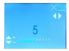
Use the Up or Down buttons to move the humidification level from 0 to 10 (0 = no humidification, 10 = maximum humidification). You will see the water droplet icons move to a higher or lower value. Once you reach the desired setting, use the Left and Right buttons to toggle to the green checkmark, if it's not already highlighted, then press the Center button to save your settings.
