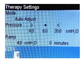
Push the Up or Down button to move the value from 0 to 3. A setting of 0 provides no exhalation relief, 3 provides the greatest exhalation relief. Press the Center button to save your selection.
