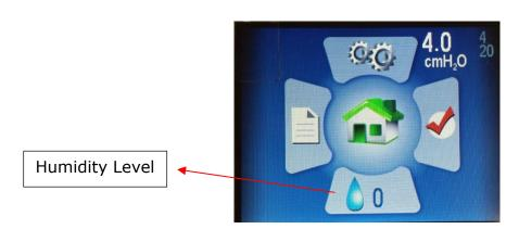
From the home screen, push the Down button to highlight the Humidifier section. Push the Center button to select it.
