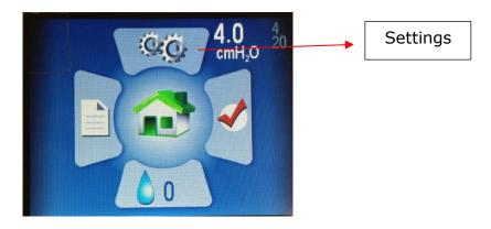
Enter the Settings screen by pushing the Up button to highlight the icon, then press the Center button to select it.
