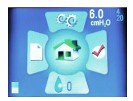
After the 30-minute drying cycle, the blower will turn off and the device will automatically enter Standby Mode. Dry mode flushes your CPAP device, tubing and mask of any residual moisture left from a therapy session.
