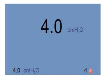
The red droplet indicates that the humidifier is not active. Normal CPAP therapy is not affected. This can be caused by any one of the following:
